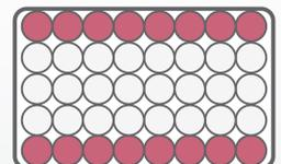
○線径1.9mm ●線径2.05mm
